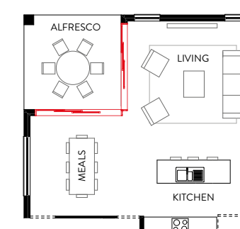
CORNER STACKER DOORS • Two 2.1 x 3.1m stacker doors
