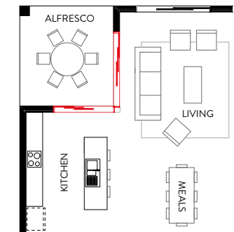
CORNER STACKER DOORS • 21-27 SSF & 21-22 SSF
